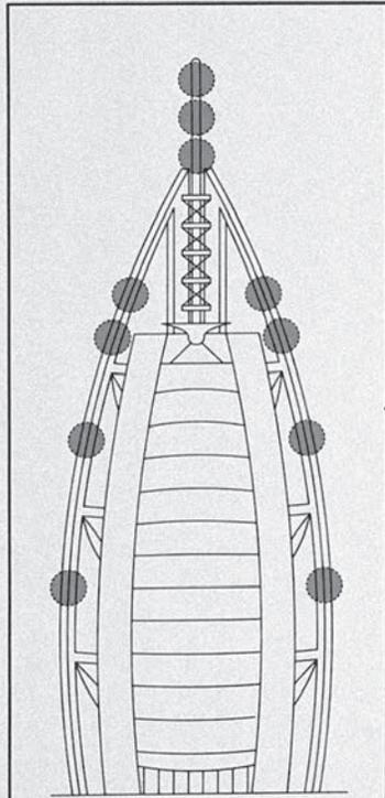
Hanging weights were installed that swing in high winds, dampening vibrations and making the building safe.
